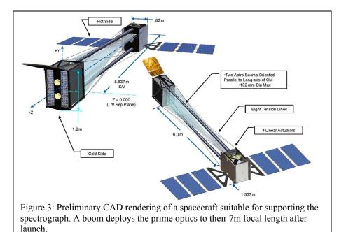
To achieve the required resolution. the system must be dispersive, there must be optics of appropriate resolution, and a system of adequate focal length to support the dispersion. To obtain the needed high collecting area, a sufficient area of xray optics must be packed into the envelope without exceeding mass constraints for launch.
