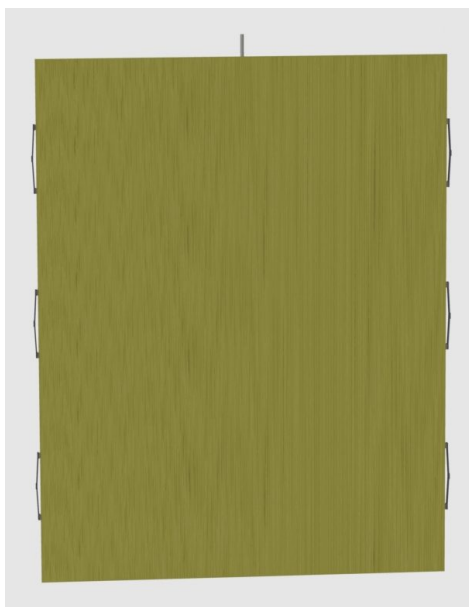
Figure 18. The mechanical design of the grating substrate with flexures bonded to the edges. These flexures are used for bonding the gratings to the carbon-fiber inserts shown in Fig. 17.
