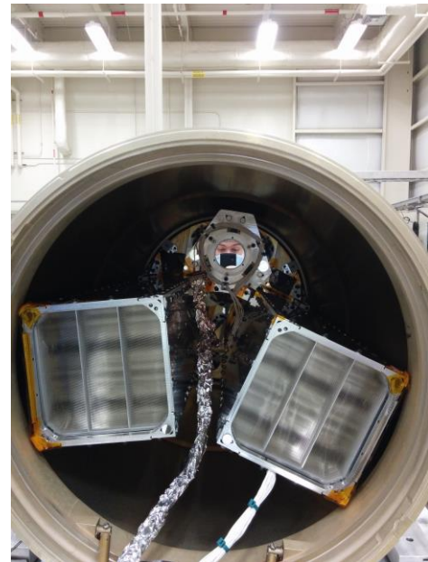
Figure 3: A view looking down the OGRESS passive focusers. To traverse the focusers, photon paths are limited to a specific angle, as can be seen in the dark line areas of each focuser. In this image, the star tracker's mass model is installed and the primary tracker's mass model is reflected in the alignment flat.
