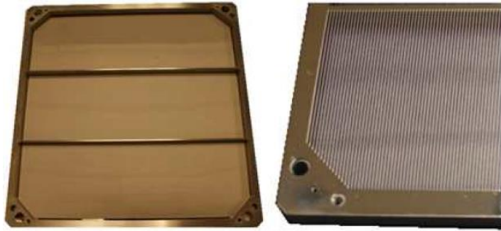
Figure 1: A single wire-grid plate bonded to its thick aluminum frame. In the zoomed image, we can see the individual wires and the slits between them.
