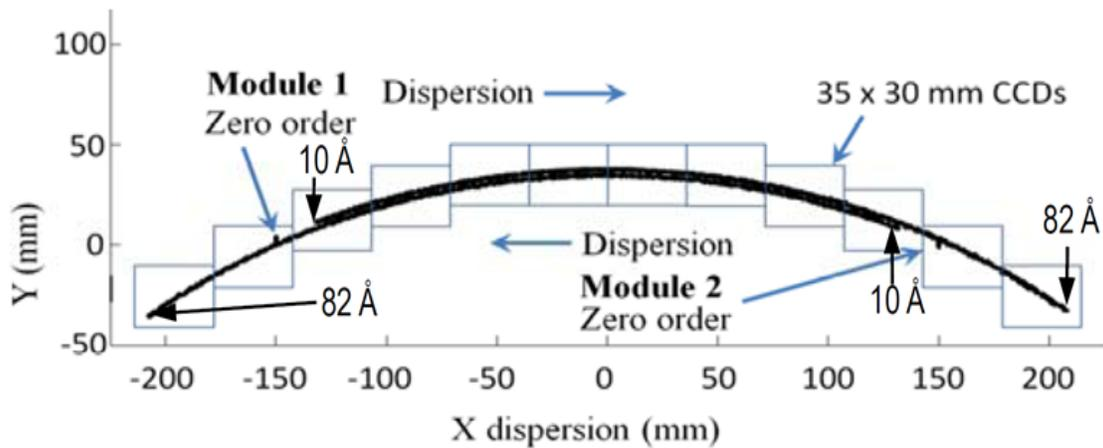
Figure 11: A raytrace of the spectra is shown overlaid on the proposed CCD array. Two arcs, one from each module, disperse in opposite directions. This allows for spectral redundancy.
