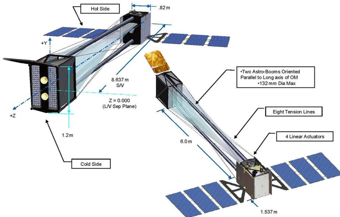
Figure 5: Spacecraft concept for WHIMex. On the left side the Optics Module is pointed out of the page.
