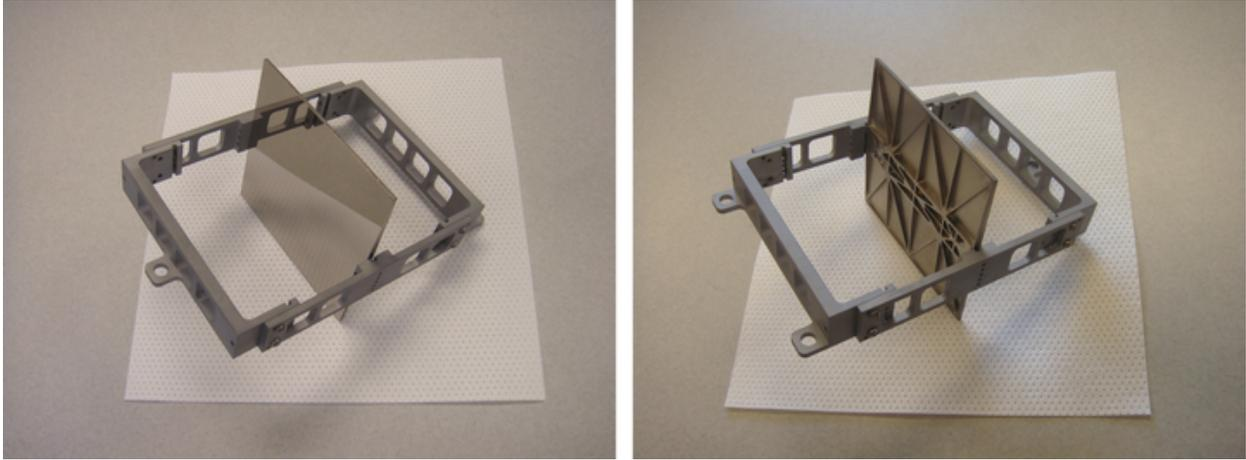
Figure 4: A high fidelity Be grating substrate assembled with a Be grating module mount. The image on the right shows the polished reflective surface while the image on the left is the lightweighted back side.
