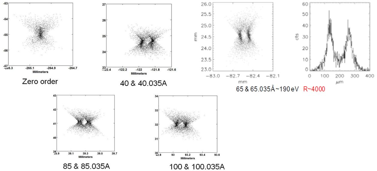
Figure 10: Spot raytraces at various wavelengths. Each pair of spots is separated by  $0.035 \text{ \AA}$ . Each set of spots is clearly separated by  $> 2$  resolution elements leading to resolutions of  $>4000$  around the blaze wavelength and longward.
