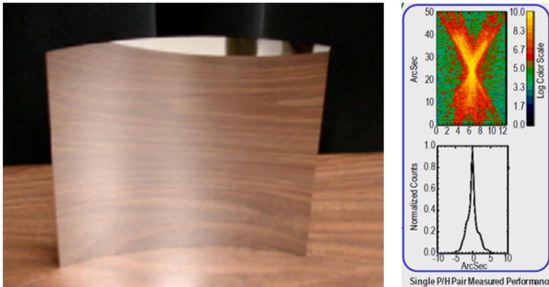
Figure 8: Left - Precision optic formed through glass slumping during the IXO program. Right – test results from a permanently bonded P/H pair mounted in a housing simulator. The telescope HPD is 9.7” at 4.5 keV with a 1.4” subapertured FWHM.
