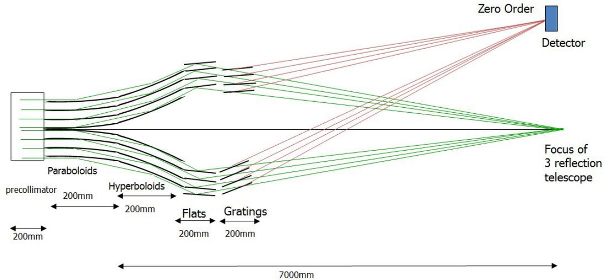
Figure 6: Schematic of the optics module. The module consists of a parallel stack of P/H pairs, followed by an array of steering flats and ultimately an array of gratings. The gratings disperse the spectrum orthogonal to the plane of the page onto an array of CCD chips.
