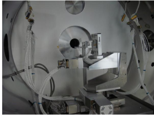
Figure 2: Test grating in the University of Colorado X-ray Test Facility (left) and in the University of Iowa Facility (right).
