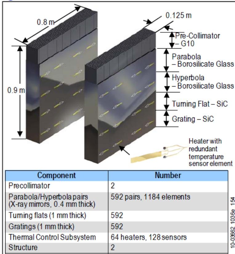
Figure 7: A CAD model of the Optics Module. The assembly consists of 2 channels of 4 reflecting optics – a parabola, hyperbola, flat, and grating. The module will operate at 20° C which is maintained by the Thermal Control Subsystem.
