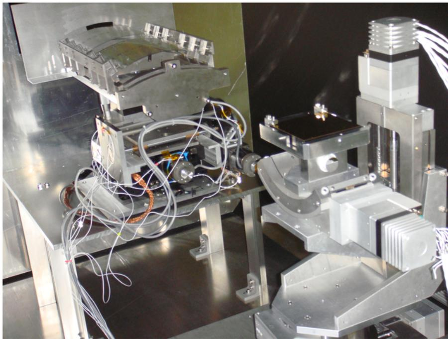
Figure 3: The MSFC Stray Light Facility large vacuum chamber with test optics. In the upper left of the image a single parabola and hyperbola are held in a kinematic mount. The test grating apparatus is located on right side of the image with 4-axis motion control.
