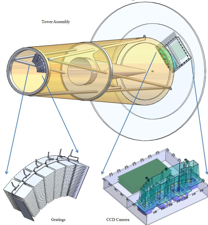
Figure 1: Schematic of the OP-XGS concept design. Six grating modules are placed on a tower assembly extended from the instrument platform which also houses the readout CCD camera.
