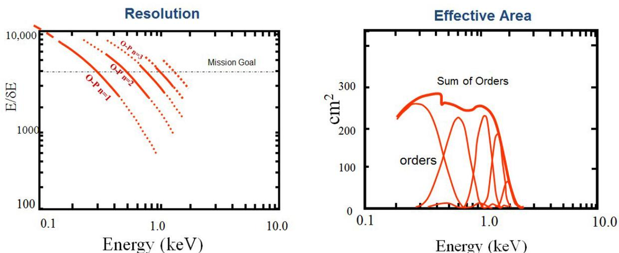
Figure 9: Expected performance of WHIMex based on detailed raytrace analysis.
